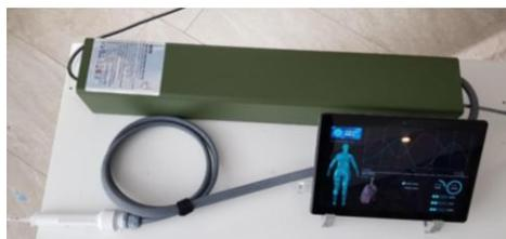
The ventilator is equipped with a mucus drainage system if the patient is in a very critical medical condition.
