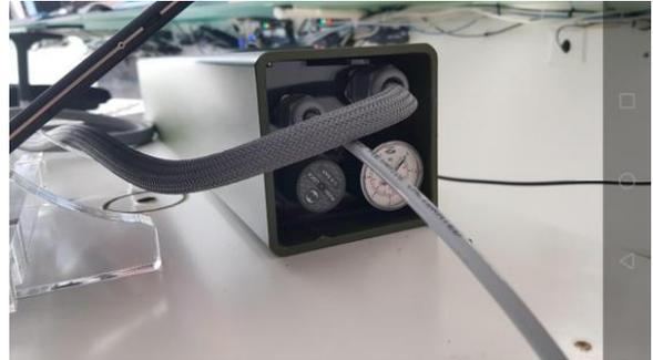
The MGPV medical device is an extremely innovative system that differs from traditional lung ventilation. In fact, it does not use mechanical systems for closing and opening the valves, but patented dynamic flow valves. There is no movement of mechanical parts inside the medical device, except for the solenoid valves.
